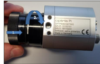
Figure 13: Inserting the lens
