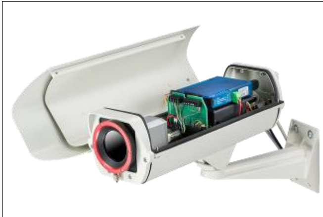
Figure 20: Outdoor protective housing for PI camera, USB server and industrial PIF
